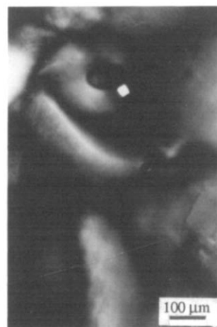
Figure 1 Schlieren texture formed in the cellulose solutions: solvent composition 24.5/75.5; cellulose concentration 14 g per 100 ml; DP 450
